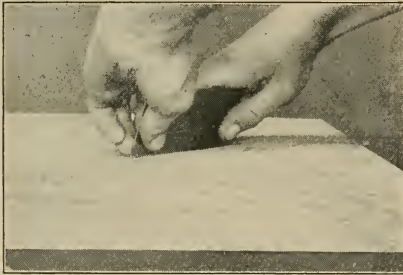
Fig. 176—Using Scraper, Pulling
